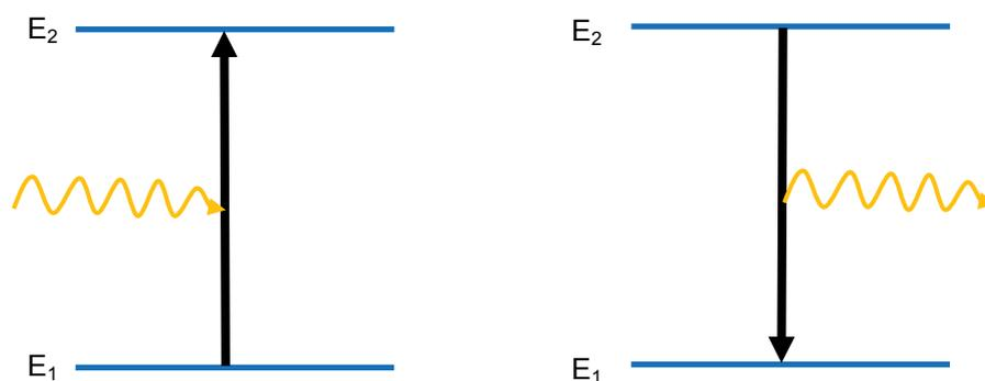
**Figure 5.18:** Schematics of absorption (left) and emission (right) spectroscopy as energetic transitions between energy eigenvalues  $E_1$  and  $E_2$ , involving either absorption or emission of light of energy  $\Delta E = E_2 - E_1 = h\nu = h\frac{c}{\lambda}$ .
