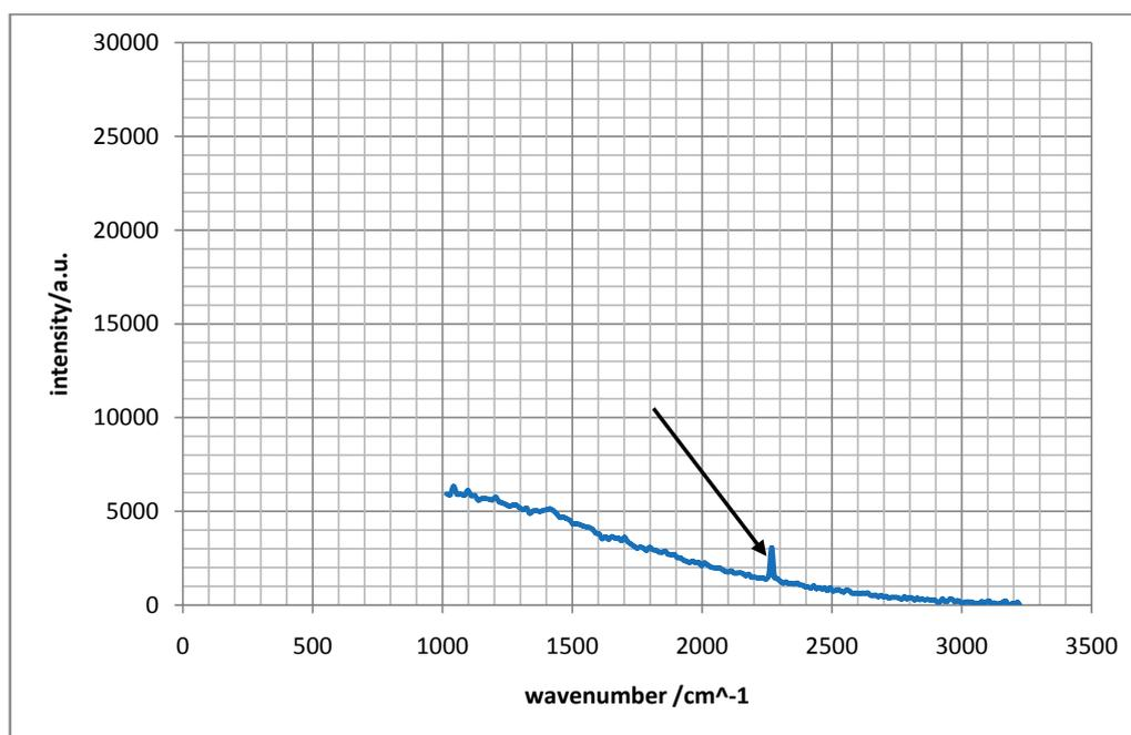
**Figure 5.23:** Raman-spectra of  $\text{CHCl}_3$  (top) and  $\text{CDCl}_3$  (bottom) showing the isotope effect (see peaks at highest wave number as indicated by arrows). Both spectra were measured with an iRaman-spectrometer by W. Schärtl at university Mainz, Germany, August 2013.
