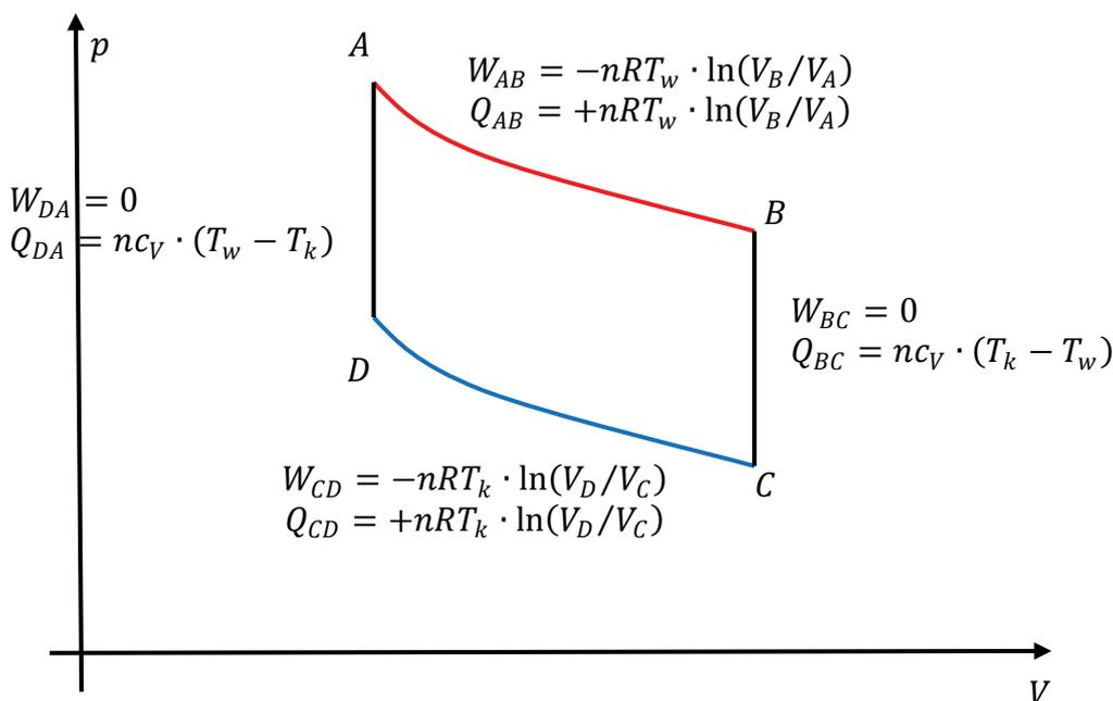
Fig. 2.10: p-V- circle of the Stirling process
