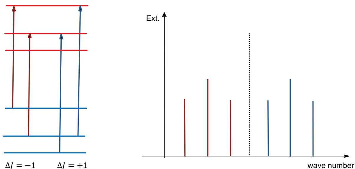
**Figure 5.22:** Energy transitions (right) and corresponding rotational-vibrational spectrum of HCl (left). Dotted line corresponds to the hypothetical transition  $\Delta J = 0$  not found in the HCl-spectrum.
