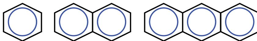
**Figure 5.10:** Particle in a box model and the  $\pi$ -electron system in condensed aromatic rings. The “box dimension” increases from benzene (left) to anthracene (right), and accordingly the absorption spectrum is red-shifted.
