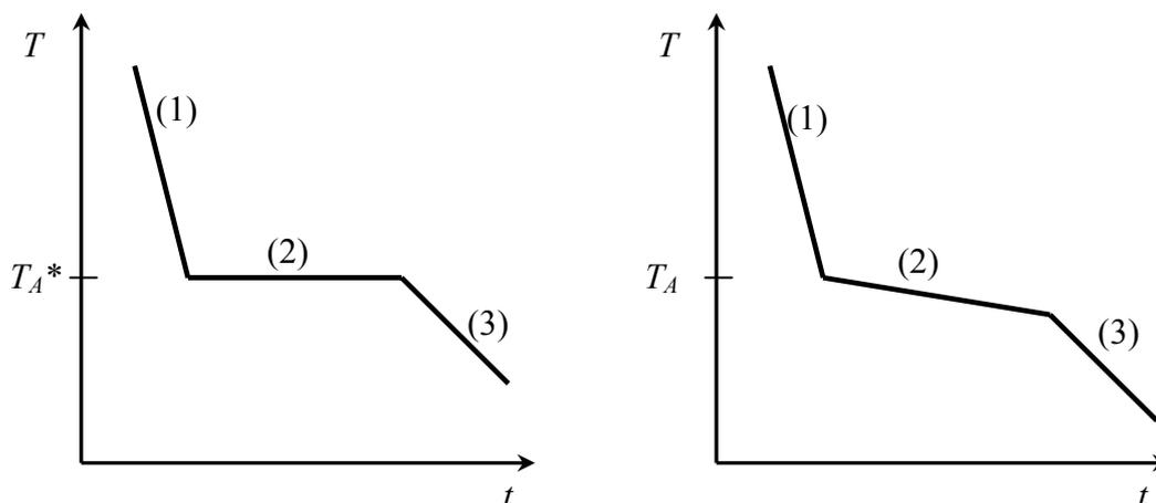
**Fig. 2.24:** Experimental cooling curves of pure liquid (left) and a binary mixture containing only one crystallizable component (right)
