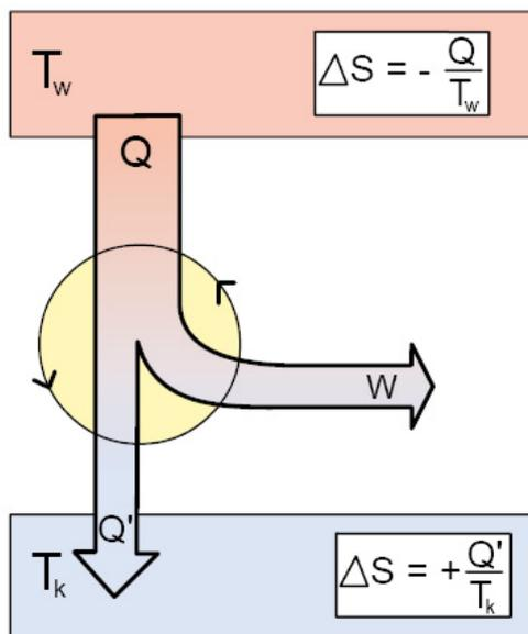
Fig. 2.7.: thermodynamic machines – principle of the Carnot process
