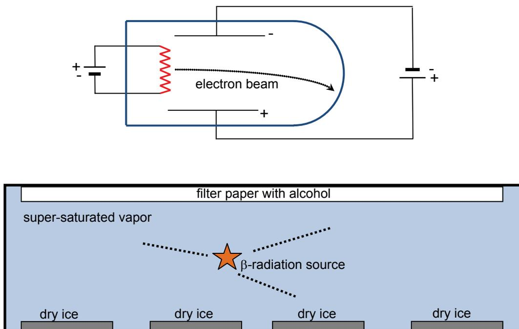
**Figure 5.1:** Cathode radiation and deviation of the electron beam in an electric field proving the negative charge of electrons (top), and proof of its particular character (a  $\beta$ -source emits electrons!) via the Wilson cloud chamber (bottom)
