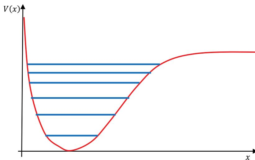
Figure 5.15: Morse potential and resulting energy levels
