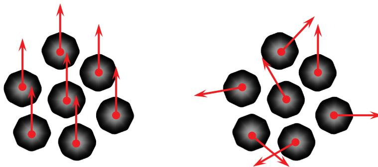
**Fig. 2.13:** difference of work (left) and heat (right), and the 2<sup>nd</sup> law of thermodynamics. Note that, if the gas is expanding in one direction (= volume work), during this process a regular flow of the particles in this direction is needed. In contrast, if the gas is heated at constant volume, only the velocity of the irregular motion of the gas particles is increasing.
